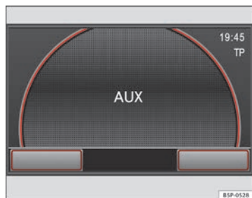
Fig. 28 External audio source connected to AUX IN multimedia socket.
