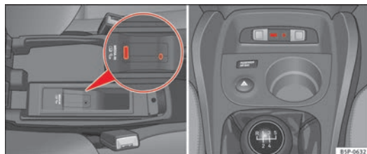
Fig. 38 MEDIA-IN socket for Altea and Leon
